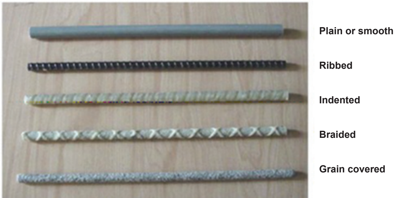
Fig. 1.2 Different Surface Characteristics of FRP bars (Abedini et al., 2017)
